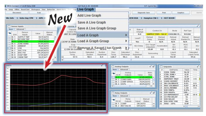
When you connect to a controller, open a MCS-CONNECT work space, you have the ability to load a saved 'LIVE GRAPH' and view it 'LIVE' in your status screen.
