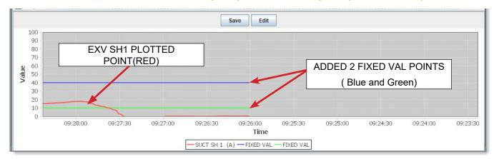
■ 'FIXED VAL' - When adding a new Live Graph you now can set 'Fixed Val' for setting up you zones for plotting a point. Each new Live Graph can contain 2 fixed values on the graph. These fixed values or lines help in seeing the movement of the plotted point (see above screen shot).
